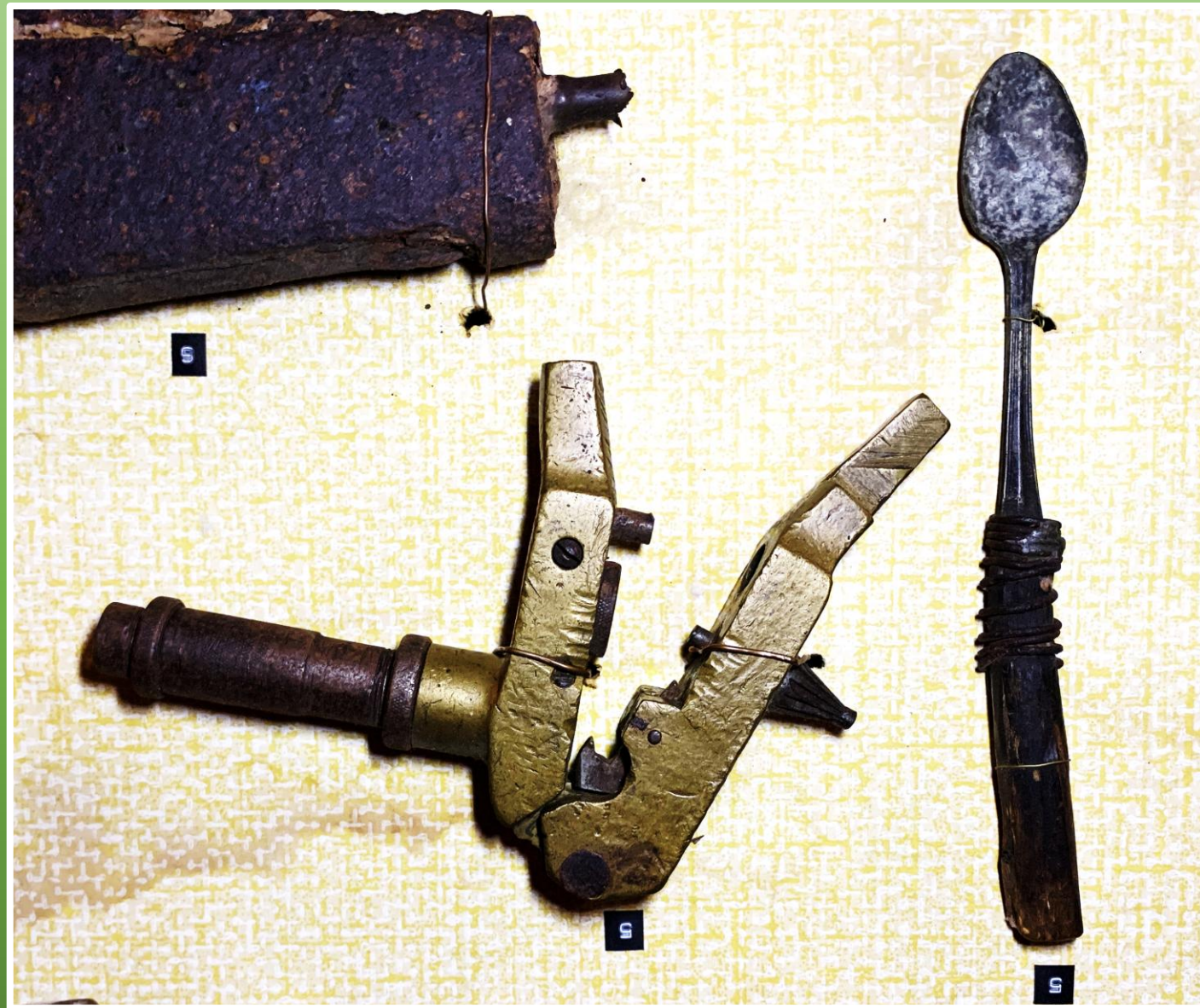
Modified bullet mold (reloader) and lead spoon. Note the handles were cut off (the brass was reused for other items); just enough handle was left to use the bullet mold.
